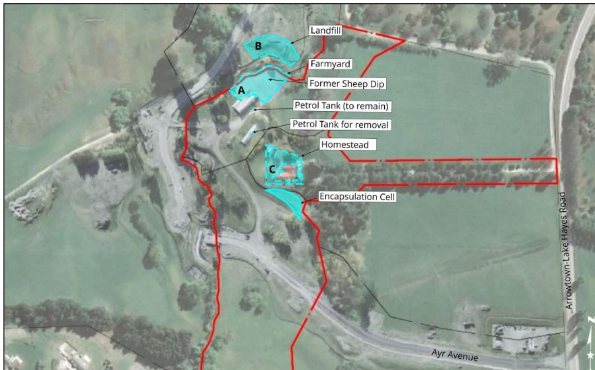
Figure 6: Aerial illustrating the three areas of remediated contamination and the location of the encapsulation cell
