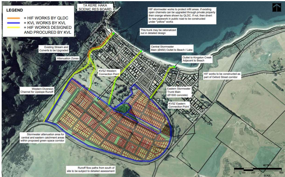
Figure 14: Proposed stormwater infrastructure for Kingston
